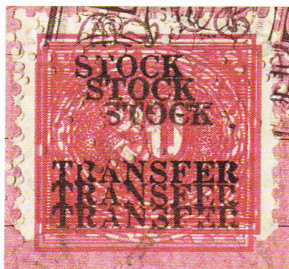
Figure 4. Overlay of transparencies of images having different indentations. The images are of the same magnification and the left edge of the word "TRANSFER" is aligned. The images are vertically shifted so that the variation in indentation is more easily observed in the overlay.
