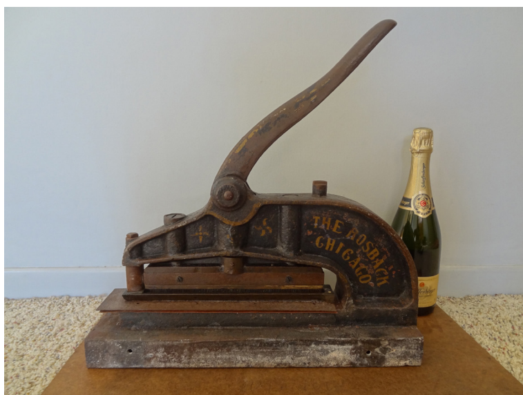
Figure 2. A Rosback Co. tabletop perforator believed to be one of their earliest, pre-1890 products. It weighs 40 lbs and requires a force of 50–80 lbs to punch the 10 inch row of pins through one or a few layers of paper. It is gauge 12 and has an average hole size matching the fake extra perforations. By using more than one layer of paper, the sharpness of cut also matches the fake extra perforations. A 0.75L bottle of champagne is shown for size reference.
